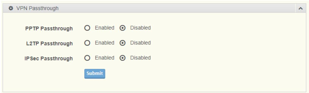
**Figure 2.16 Networking > Security > VPN Passthrough.**
