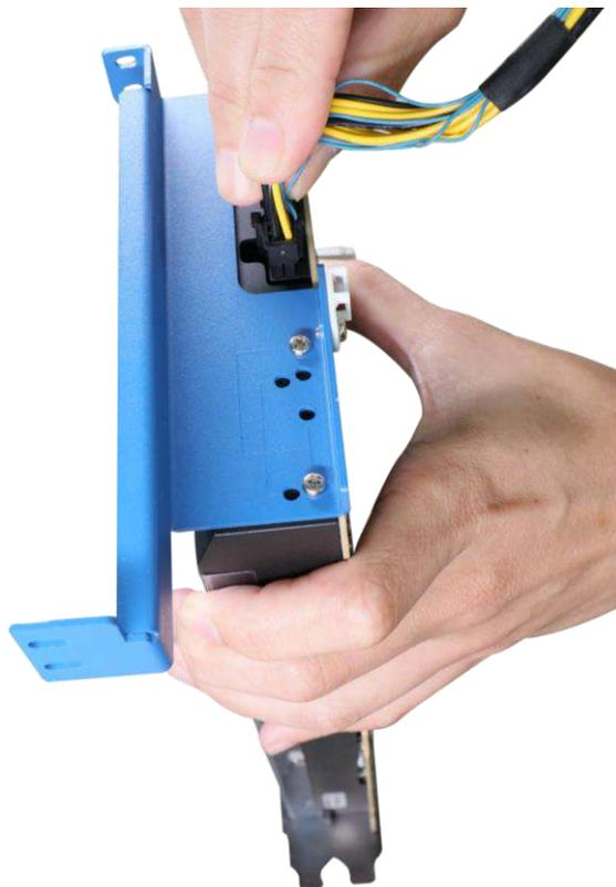
7. Gently lower the graphics card into the PCIe slot while ensuring the gold-fingers are inserted, the graphics card panel is properly inserted and secured with screws.
