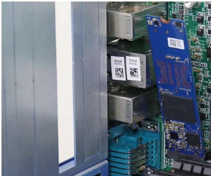
4. Gently press down and secure the module with an M2.5 P-head screw.
