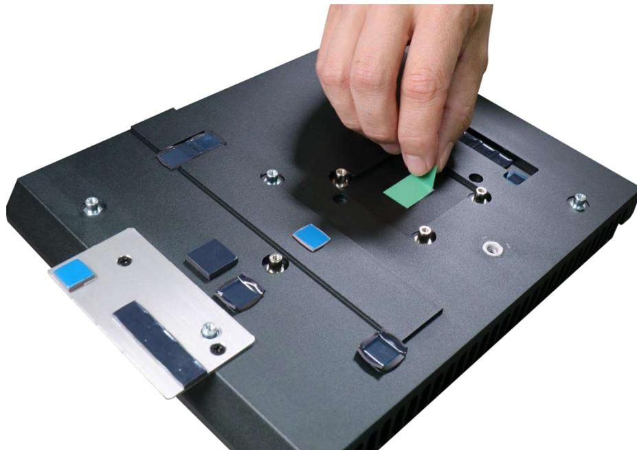
7. With the four motherboard standoffs aligned, gently lower the motherboard onto the heatsink and secure the four screws.
