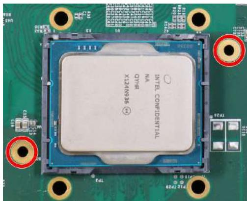
**Screw holes for CPU retention bracket**
