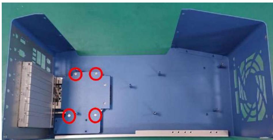
3. Turn the bracket upside down and secure the tray's chassis onto the bracket by inserting screws inside-out.
