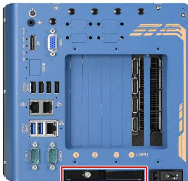
2. You may insert and install the HDD/ SSD without disassembling the enclosure. Simply lift to spring open the lever to gain access to the hot-swap slot.
