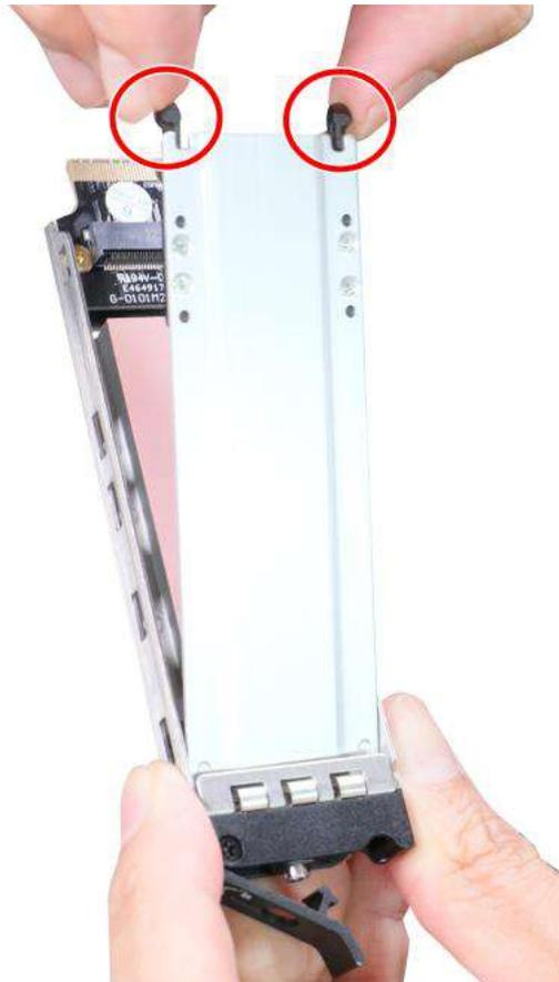
8. Insert the NVMe SSD module on a 45° angle and secure with a screw.
