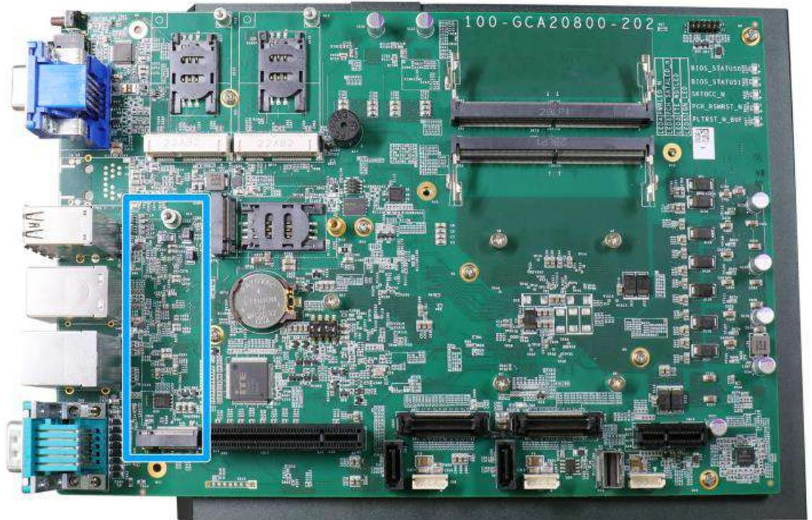
The system has a Gen4x4 PCIe M.2 2280 slot for you to install an NVMe SSD for the ultimate performance. The NVMe SSD offers noticeable performance advantages over 2.5" SSDs for smoother operating system operation and responses.
