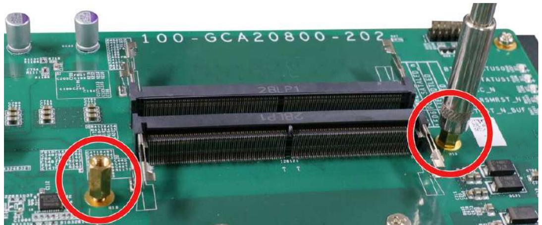
**Remove the copper stands supporting the memory module's heatsink**
