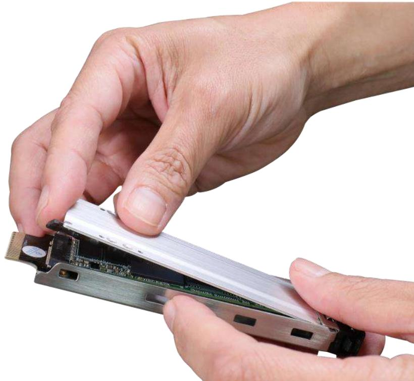
11. Insert the tray with the installed NVMe SSD back into the enclosure, and push the lever back in to complete the installation. The tray is also lockable with the provided key when you purchase this optional kit.
