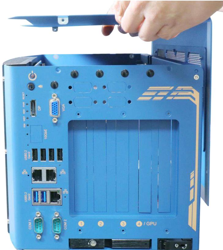
**Place L-shape side panel onto the enclosure**
