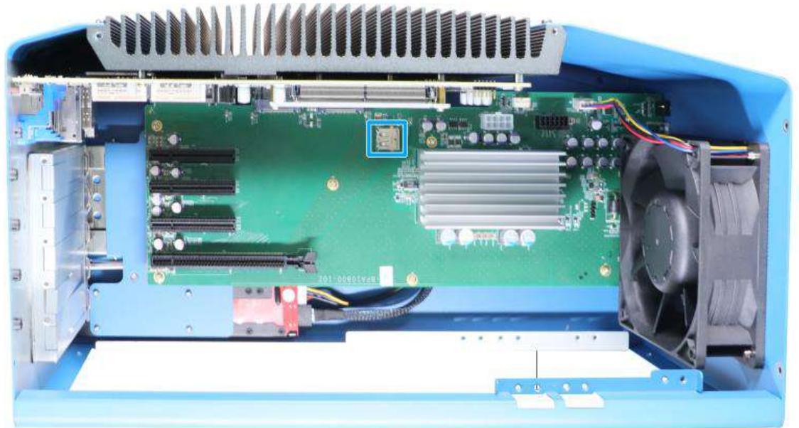
The system's daughter board has an internal USB2.0 port on the PCBA. You can utilize this USB port to connect a USB protection dongle inside the chassis of the system.
