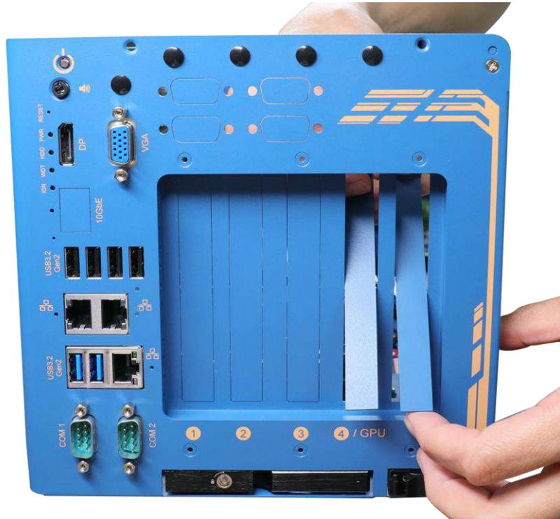
4. Take out the graphics card dedicated bracket and cable and attach the cable sorting peg.
