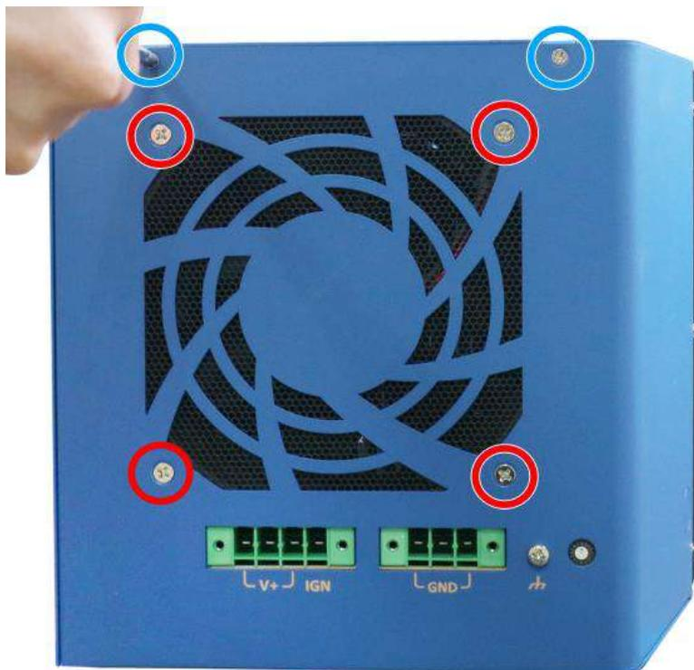
5. Gently lift the L-shape cover panel to separate it from the enclosure.
