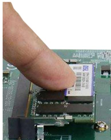
**Press module down to clip into position**
