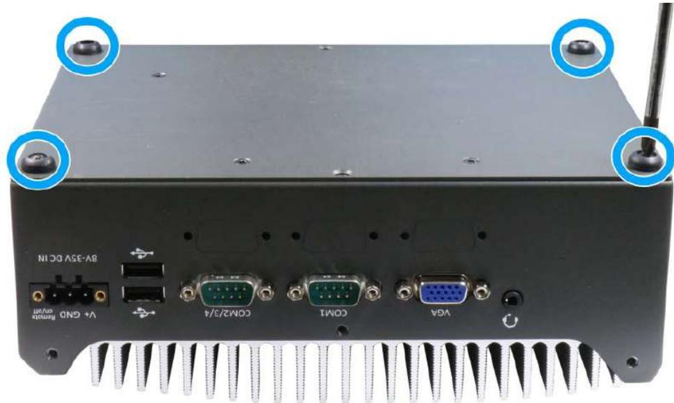
10. Gently lift and remove the bottom panel to access the hard drive cage and SATA/ power connectors on the motherboard.
