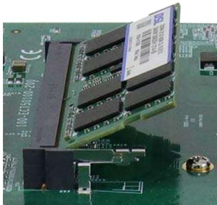
**Insert module into slot**
