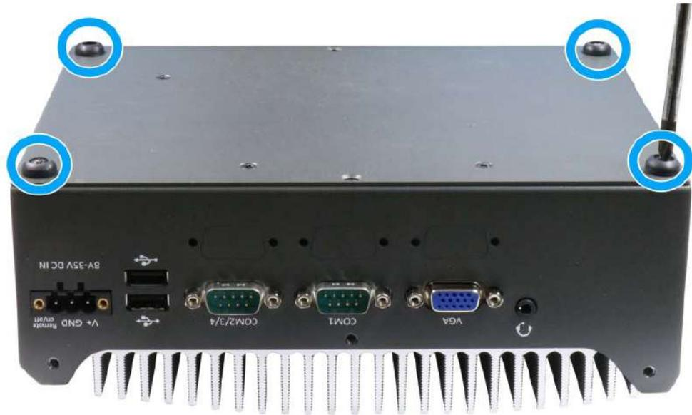
2. Gently lift and remove the bottom panel to access the hard drive cage and SATA/ power connectors on the motherboard.
