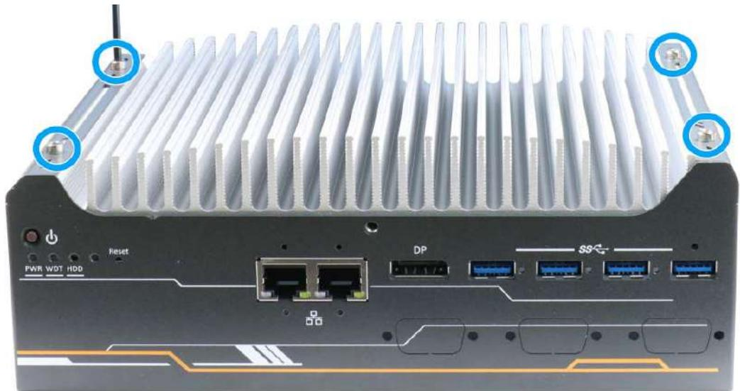
4. Unscrew the four (4) screws at the bottom of the system.
