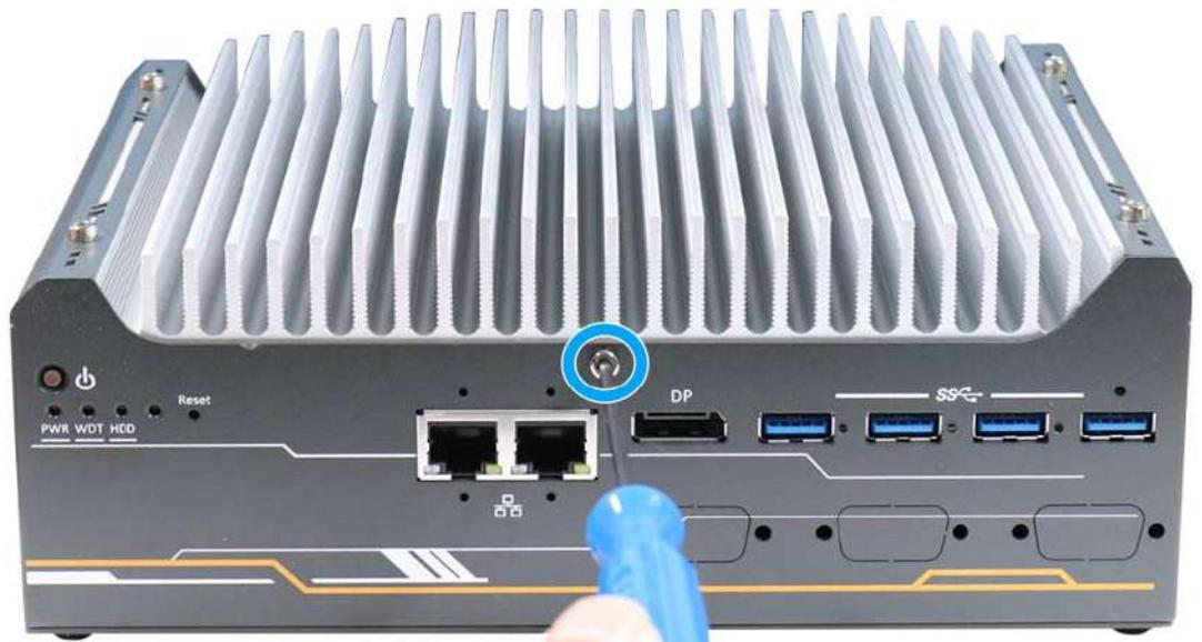
3. Unscrew the four (4) screws on top of the heatsink.
