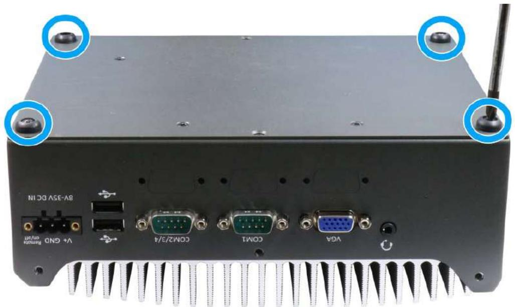
5. Gently lift and remove the bottom panel.
