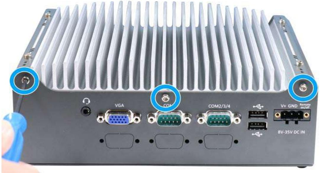
2. Unscrew the screw indicated on the panel shown below.
