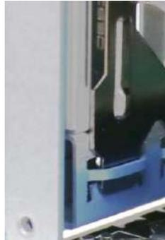
**Make sure bezel panel is inserted properly**
