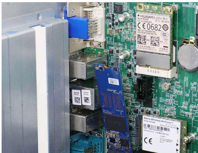
4. Gently press down and secure the module with an M2.5 P-head screw.
