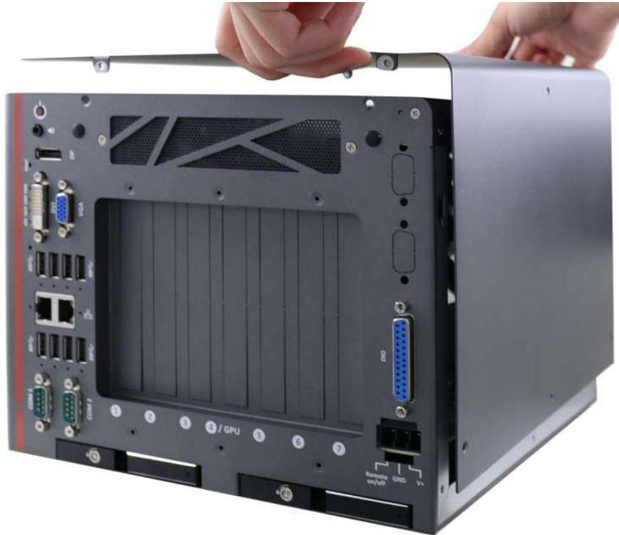
Place L-shape side panel onto the enclosure
