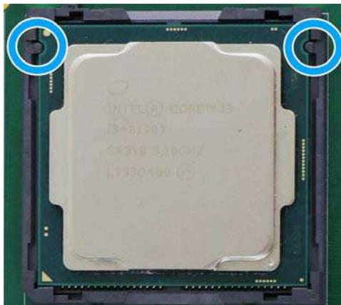
4. Locate the CPU retention bracket from the accessory box. Place the retention bracket on the CPU and hold it in place.
