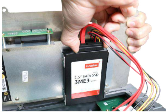
Disconnect the SATA/ power connector
