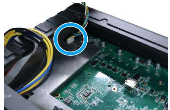
Unplug the 4-pin ATX connector
