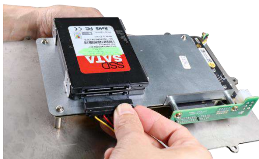
Connect the bottom hard drive first
