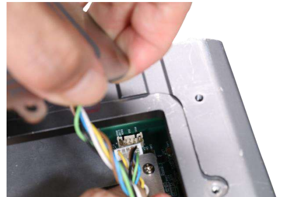
Connect from the motherboard side
