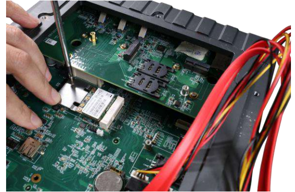
Secure the module with a screw
