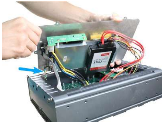
Connect the 4-pin power connector
