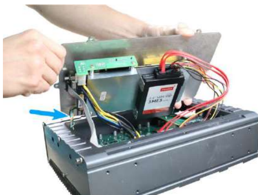
Disconnect the 4-pin power connector
