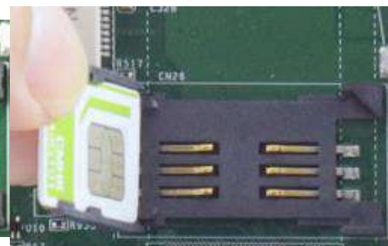
Insert SIM card with pins facing up
