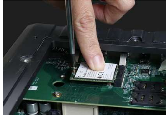
Secure the module with a screw
