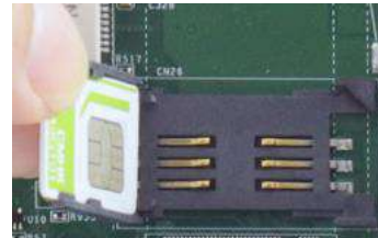
Insert SIM card with pins facing up
