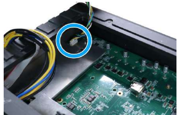
Unplug the 4-pin ATX connector
