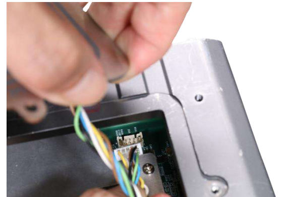
Connect from the motherboard side
