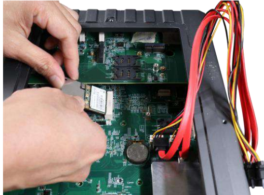
Insert into slot on a 45 degree angle
