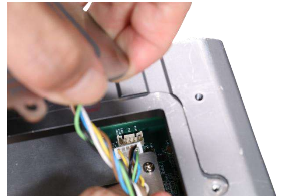
Connect from the motherboard side
