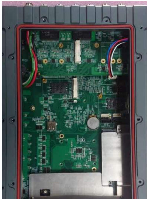
O-ring seated properly in the groove
