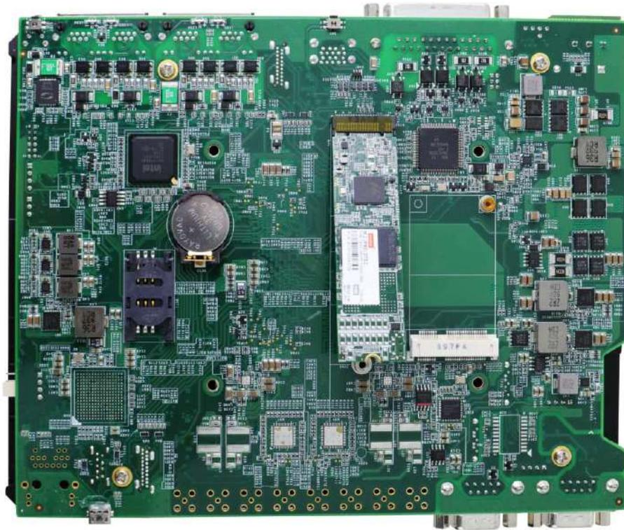
4. Gently push it towards the motherboard and secure the NVMe SSD with the supplied screw.
