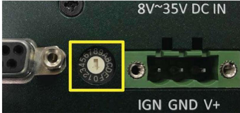
2. Connect the 3-pin terminal plug.
