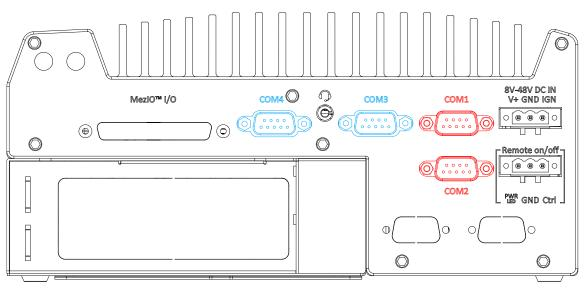
The system provides four COM ports for communicating with external devices. These COM ports are implemented using industrial-grade ITE8786 Super IO chip (-40 to 85°C) and provide up to 115200 bps baud rate.
