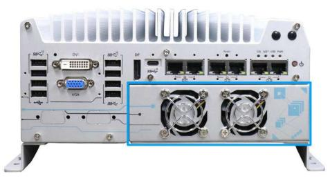
The Cassette module compartmentalizes the heat generated and effectively manages thermal conditions of both the system and graphics card. The modular design reduces the complexity of installing and replacing graphics cards in the fanless controller. In addition, the mechanical design creates a sealed wind tunnel to bring in cold air and expels hot air via system fans to offer the system extreme stability and reliability.
