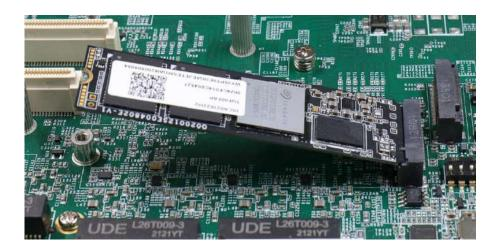
2. Insert the module on a 45 degree angle.
