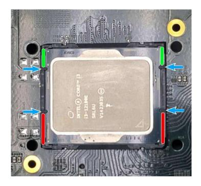
6. Locate the CPU retention bracket (holder) from the accessory box. Place the retention bracket on the CPU and hold it in place. Make sure the indicator triangle engraved on the CPU's integrated heat spreader (HIS) and the triangle indicator on the retention bracket are positioned in the same corner (indicated by blue circles).
