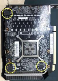
For MSI and PNY graphics cards, stick the two 36x6x6mm Poron-Cs onto the Cassette module cover
