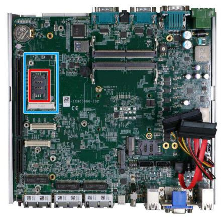
Before installing the mPCIe module, you need to insert the Mini-SIM card. Slide the SIM slot holder and lift the SIM card holder. Insert the Mini-SIM card (pins facing up), shut the SIM holder and slide it to lock the SIM card in-place.
