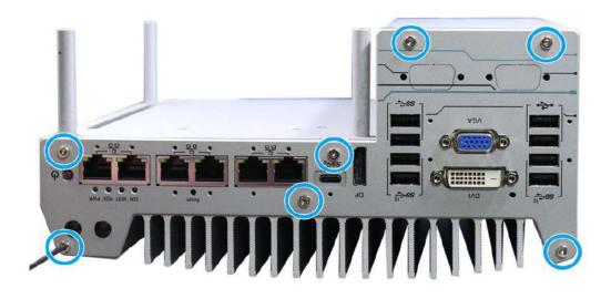
3. On the front I/O panel, remove the hexa-screws indicated below.
