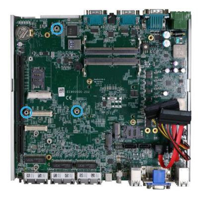
3. Gently lower the MezIO<sup>™</sup> module onto the three stand-mounts while matching the MezIO<sup>™</sup> interface. Secure the module using three screws supplied.
