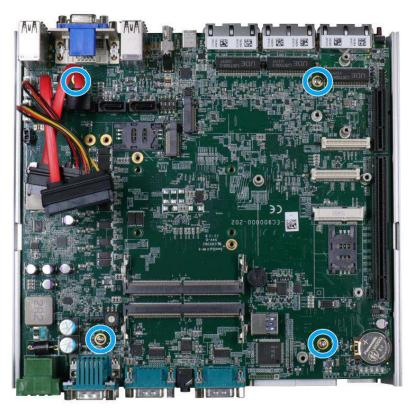
Secure motherboard with four screws
