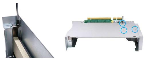
Remove the screws securing the graphics card
