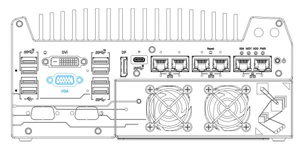
VGA connector is the most common video display connection. The VGA output supports up to 1920x1200@60Hz resolution.
