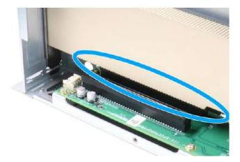
Properly inserted into the PCIe slot
