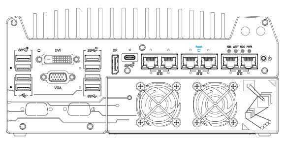
The reset button is used to manually reset the system in case of system halt or malfunction. To avoid unexpected reset, the button is purposely placed behind the panel. To reset, please use a pin-like object (eg. tip of a pen) to access the reset button
