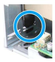
Insert and secure graphics card into PCIe slot
