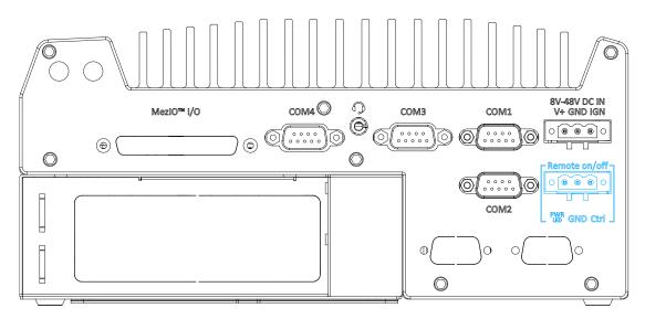
3. With DC power connected, pushing the power button will turn on the system and the PWR LED indicator will light up. Pushing the button when system is on will turn off the system. If your operating system supports ATX power mode (i.e. Microsoft Windows or Linux), pushing the power button while the system is in operation will result in a pre-defined system behavior, such as shutdown or hibernation.
