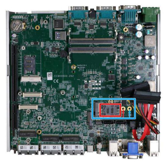
3. Insert the module on a 45 degree angle.
