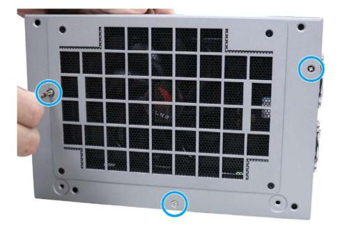
9. Place the enclosure cover, and secure the enclosure with screws indicated.
