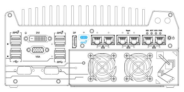
The system's USB 3.2 Gen2x2 type-C port offers up to 20Gbps of data transfer bandwidth, and is implemented via the native xHCI (eXtensible Host Controller Interface) controller. The port is backward compatible with USB3.2 Gen.1 USB 2.0, USB 1.1 and USB 1.0 devices via a USB hub (not included) to connect to external devices.
