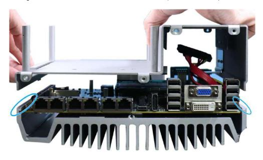
2. Install the front panel and secure screws indicated in **blue**.
