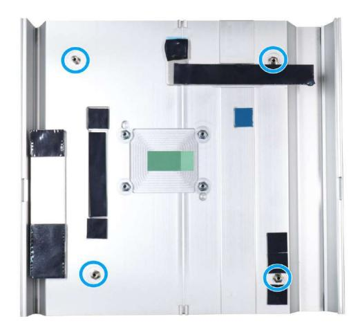
12. Once the motherboard has been installed, you're ready to secure the four screws that help the heatsink apply pressure to the CPU/ chipset die. You'll want to apply even pressure to the corners by gradually tightening each screw. Please refer to the recommended order when tightening the screws.
