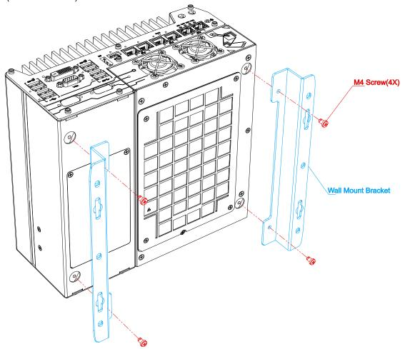
2. Place the system on a flat surface portion of the wall and secure it with four (4) M4 screws.
