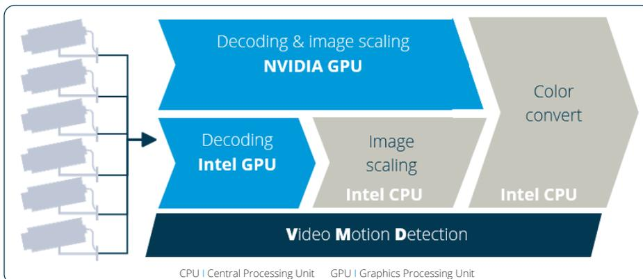
The load balancing requires no setup and is completely automatic: XProtect will first distribute the load necessary for video decoding and video motion detection (VMD) evenly between the Intel GPU (using Intel Quick Sync®) and the added NVIDIA graphics cards. Then the load will be balanced automatically according to the thresholds defined in the
