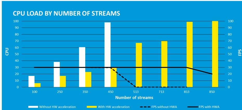
Performance measured for h.264 stream format in full HD (1920X1080). Tested hardware: Windows server 2016, 2X Intel Xeon Silver 4114, 64 GB RAM, 4X NVIDIA Quadro P2000
