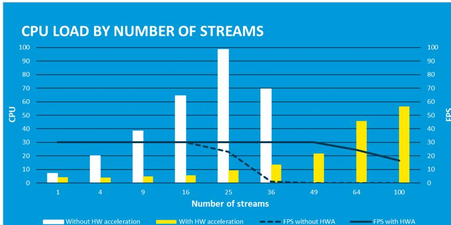
XProtect Smart Client performance measured for h.264 stream format in full HD. Tested hardware: Windows PC with Intel Core i7-8700K processor at 3.70GHz, 32 GB RAM, 2X NVIDIA GeForce GTX 1080 8GB
