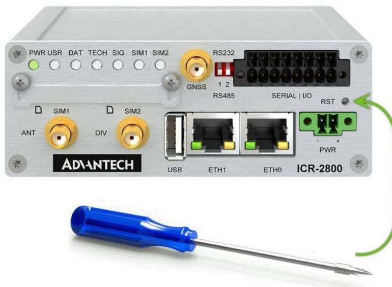
Figure 22: Resetting the Router
