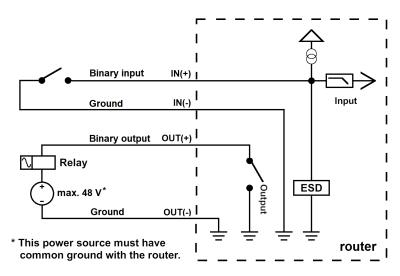
Figure 10: Functional Scheme of the Binary Interface
