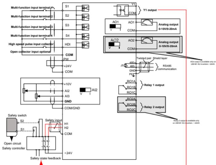
Figure 3-9 Wiring of control circuit
