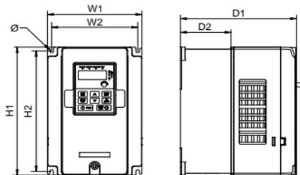
Wall mounting of 3PH 400V 4–37kW and 3PH 230V 1.5–7.5 kW inverters
