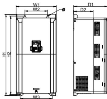
Wall mounting of 3PH 400V 45–75kW inverters
