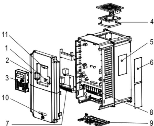
Figure 2-4 Product structure (Three phase 400V,  $\geq 4\text{kW}$ )
