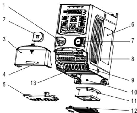
Figure 2-3 Product structure (Three phase 400V,  $\leq 2.2\text{kW}$ )
