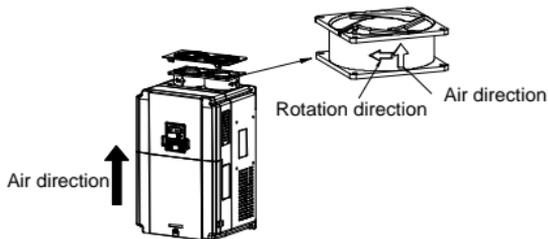
Figure 6-2 Fan installation of the inverters 3PH, 400V,  $\geq 4\text{kW}$
