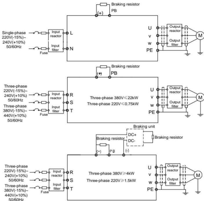
Figure 3-3 Connection diagram of main circuit
