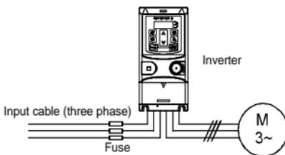
Figure 3-16 Fuse configuration
