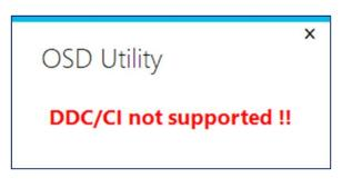
**WARNING!** The host device also requires the **appropriate graphic driver** for OSD utility to be fully operational; otherwise, the following error message will be displayed during initialization.
