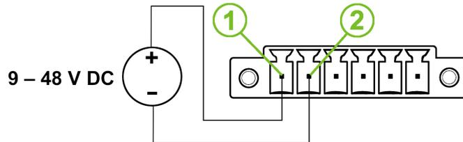
Figure 14: Connection of Power Supply
