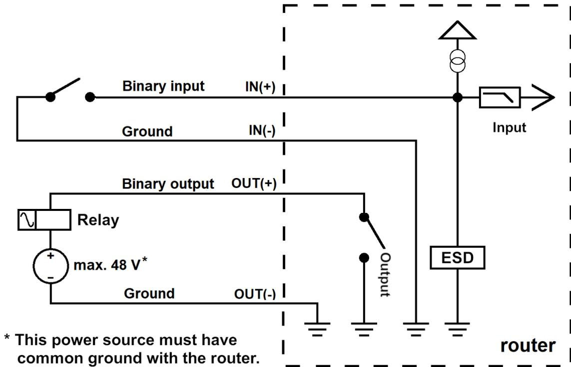
Figure 17: Functional Scheme of the Binary Interface
