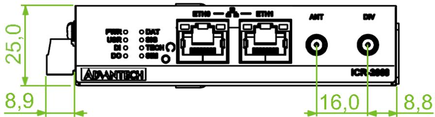
Figure 6: Router Dimensions – Front View
