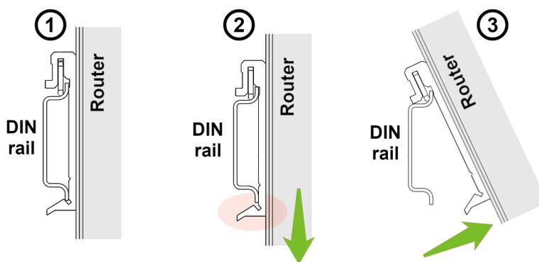
Figure 10: Removing Router from the DIN Rail
